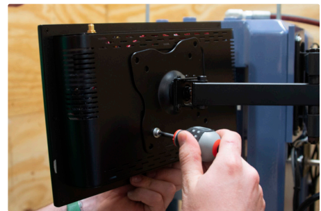
Fig. 2b: Tighten screws—do not overtighten
