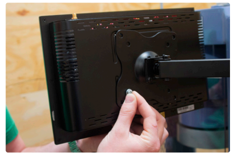
Fig. 2a: Tighten screws with fingers
